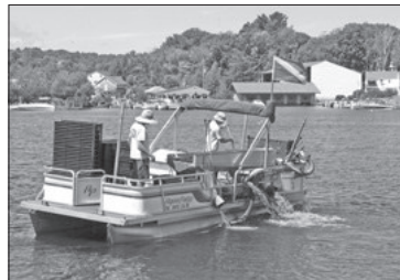
DIVER ASSISTED SUCTION HARVESTING (DASH) of milfoil took place in Back Bay on Tuesday, Aug. 14. A diver is below the surface hand pulling plants and sending them up via the harvester suction line.
